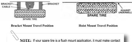
with the underside of the recreational vehicle to insure maximum road clearance and stability in travel. Raising and lowering the hoist
