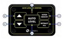
**NOTE:** Pressing both the arrow buttons simultaneously turns on the touchpad. Touchpad will time out after 7 minutes of non-use.
