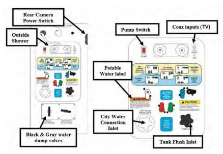
**The Uni-Doc Utility Center** is located in an exterior compartment and allows you to perform the following functions:
