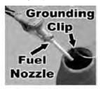
Fuel Nozzle in contact with receiving tank
