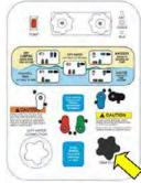
Sewer Tank Flush Inlet on Utility Center
