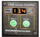
**POWER** button is used to turn the inverter on and off. To turn on the inverter and the LED display press and hold **POWER** for 1 second until you hear a beep.
