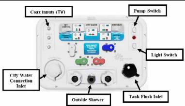
The Uni-Doc Utility Center is located in an exterior compartment and allows you to perform the following functions:
