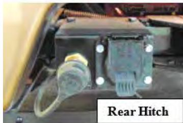
An air hose coupling (in the vicinity of the electrical harness connection) located at the rear of the motorhome supplies the air pressure to the tow vehicle controller.
