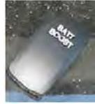
To operate, press and hold the Battery Boost start switch located on the driver’s left side console. While the battery boost switch is pressed, use the ignition key to start the chassis engine or the generator switch to start the generator. Release the battery boost switch once the engine or generator has started.
